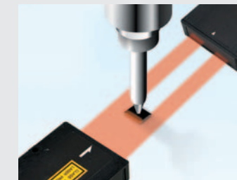
Finding a fine chip vacuumed by picker.
